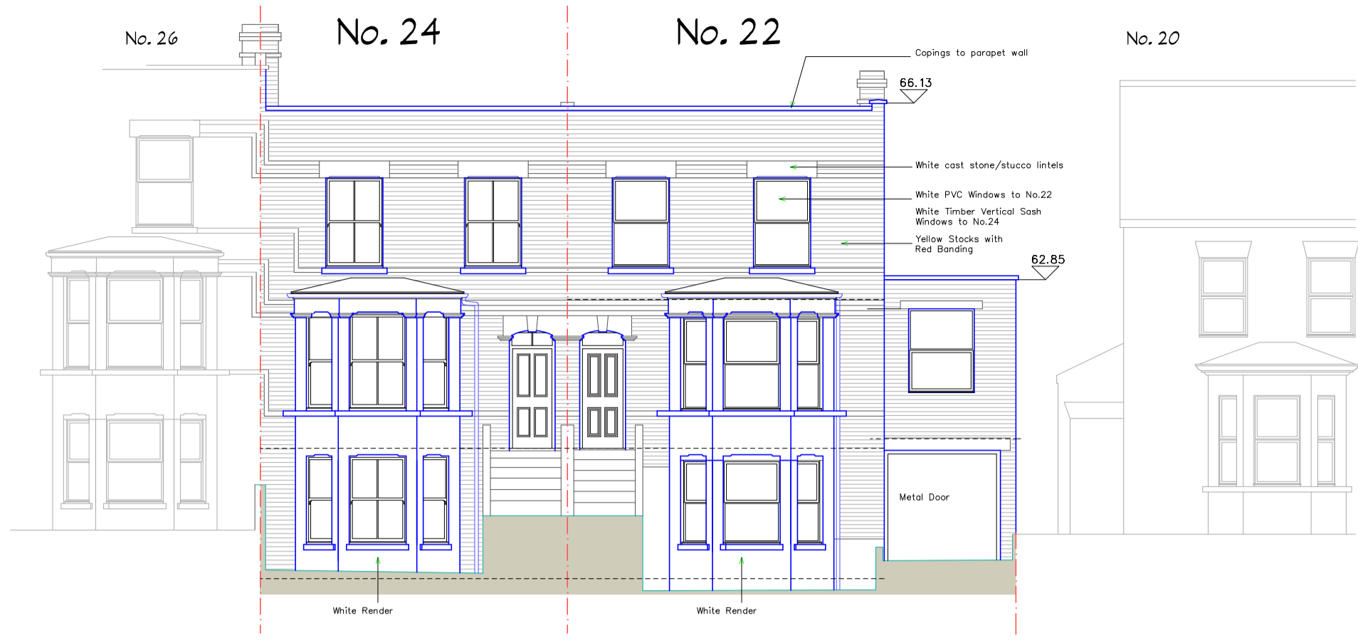
FRONT ELEVATION (North East)
